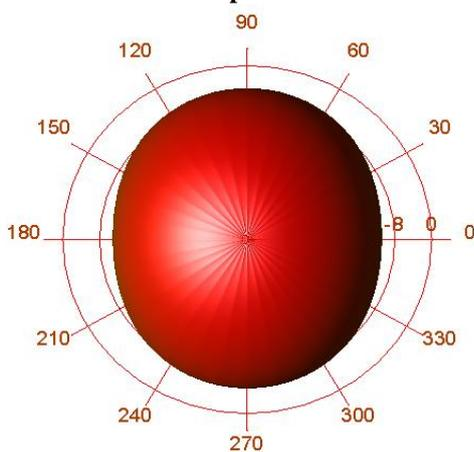
Figure 8b. 3-dimensional top view of radiation pattern
