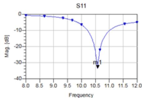
Figure 5. Plot of return loss magnitude vs frequency
