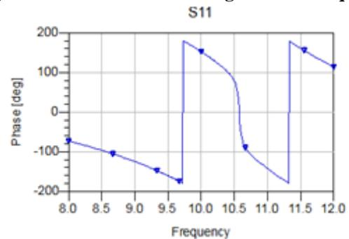
Figure 6. Plot of return loss phase vs frequency
