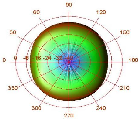
Figure 8a. 3-Dimensional bottom view of radiation pattern
