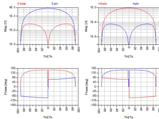
Figure 10. E-plane and H-plane radiation pattern in Cartesian coordinates
