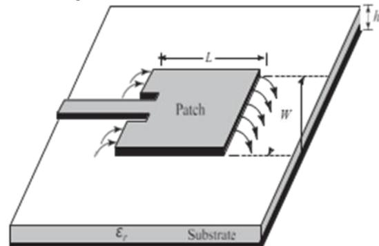
Figure 1. Microstrip patch antenna
