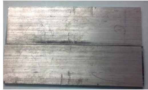
Fig 2 : 150mm X 50mm X 6mmAluminium Alloy plates
