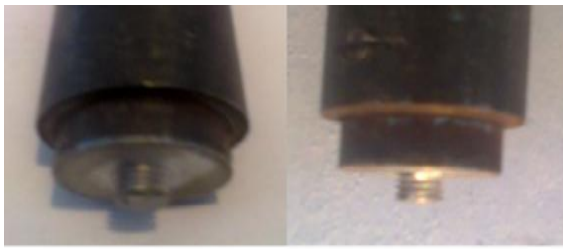
(A) PIN LENGTH 5.5 mm (B) PIN LENGTH 5.7 mm
