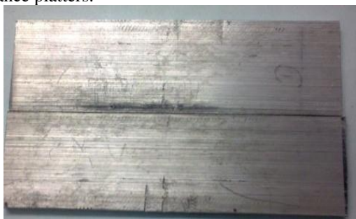
Fig 2 : 150mm X 50mm X 6mmAluminium Alloy plates
