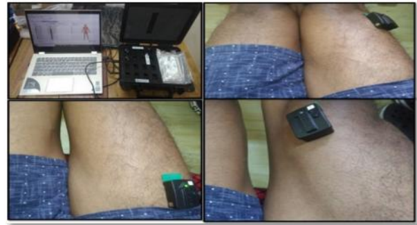
Fig. 3: EMG acquisition system and sensor positioning for limb muscles
