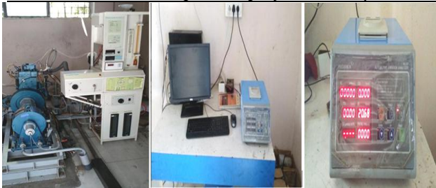
Fig.1. Actual system of Computerized SI engine Test Rig with Exhaust Gas Analyzer
