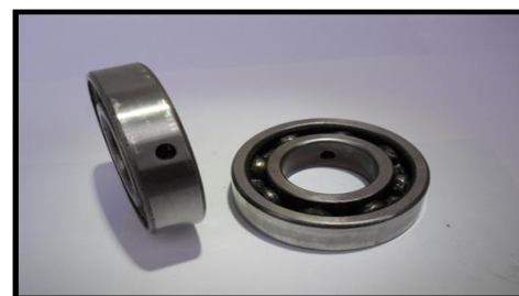
Fig.2 Bearing Specimens used in Experimental Study
