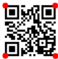
Fig. 12 Red Points indicate the Quad of a QR Code
