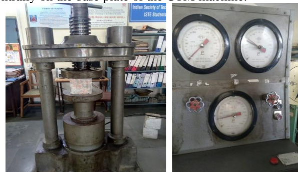
Fig. 1 Compressive strength test
