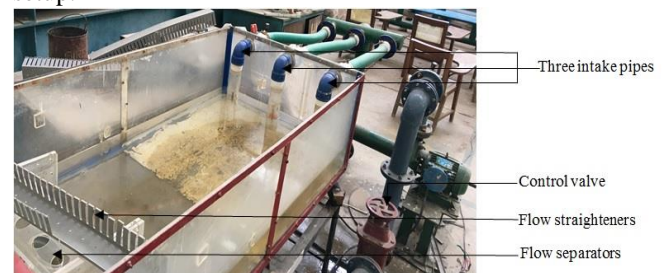
Figure 1 Experimental setup of pump intake
