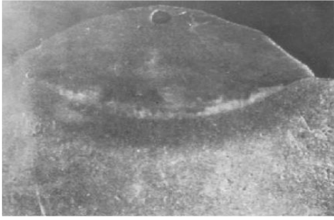
Fig.1 Macro-photograph showing proper fusion between mild steel and grey cast Iron.
