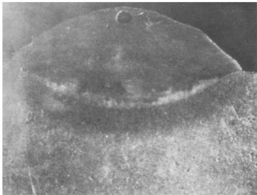
Fig.1 Macro-photograph showing proper fusion between mild steel and grey cast Iron.
