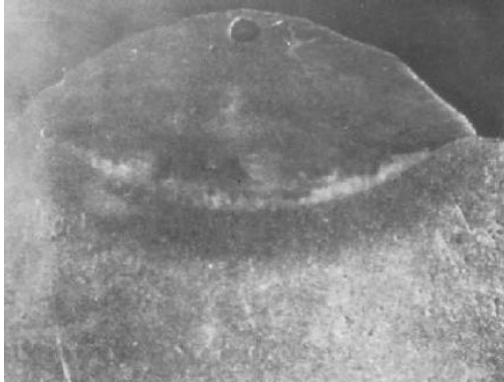
Fig.1 Macro-photograph showing proper fusion between mild steel and grey cast Iron.
