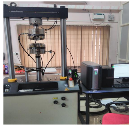
Fig. 8. Fatigue Machine Set-up
