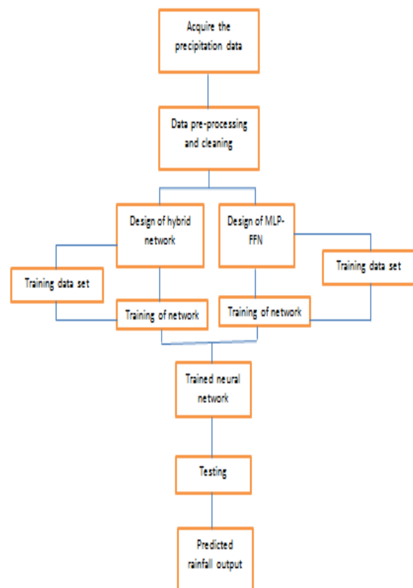
Fig 3.1 is a flowchart which explains the flow of proposed system
