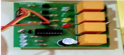
Figure 3: Relay board
