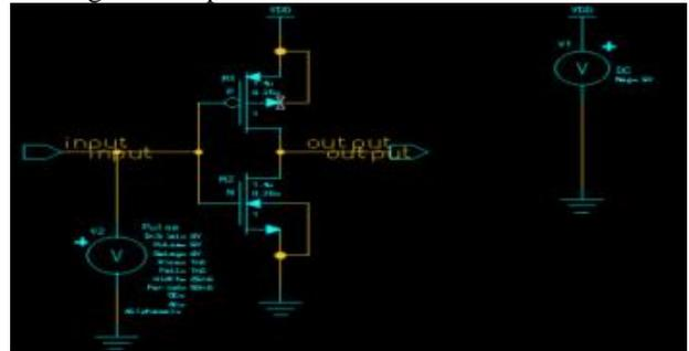
Fig.8 Schematic of Inverter of 0.35u of 1V
