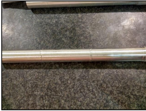
Fig. 5: 15s To 25s Workpiece Using 200mm Cutting Length
