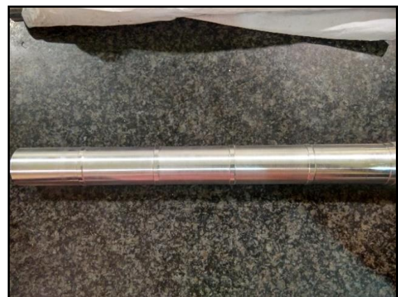
Fig. 4: 2s To 10s Workpiece Using 100mm Cutting Length
