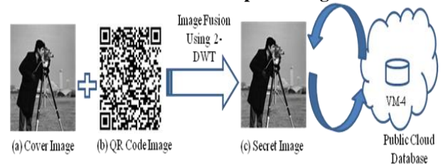
Fig. 5. The original Cameraman image (a) The Third QR code image (b) The cover fusion image stored on public cloud for further processing.
