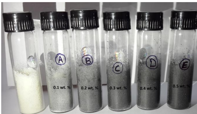
Fig 1. Photograph of pristine PCM (acetamide) and PCM-NG composite samples having different NG concentrations (0.1, 0.2, 0.3, 0.4 and 0.5 wt. %) of NG.
