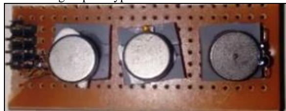
Fig. 10: Coin Vibrators module
