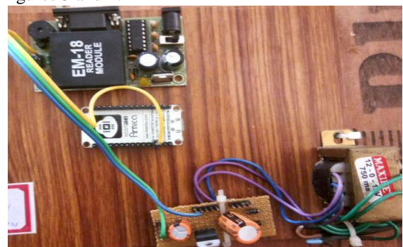
Fig.4. Node integrated with EM-18 RFID Reader Module.
