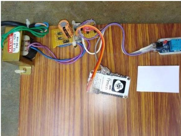
**Fig.3. Node integrated with DTH Sensor**
