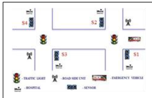
Fig. 1: Schematic representation for interconnection of RSUs and Emergency vehicles with traffic light
