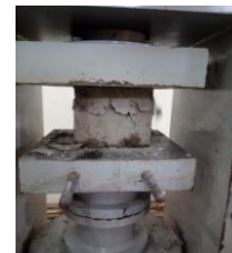
Fig 2 Compressive test on specimens
