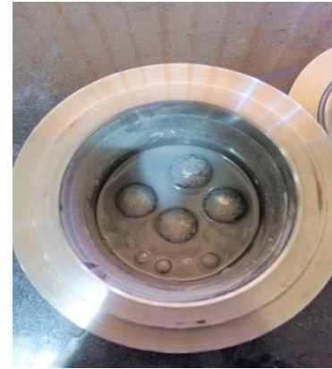
Figure 2: ball mill powder in toluene medium
