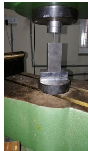
Figure 3: uni-axial compaction under UTM
