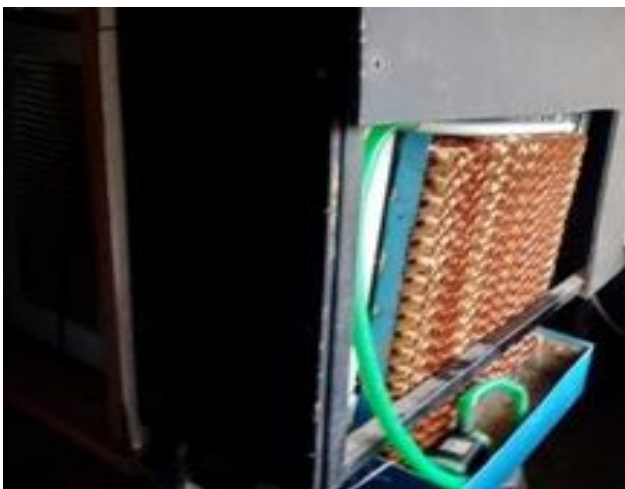
Fig.1 Evaporative cooler attached back side on condenser of Window Air Conditioning Trainer.
