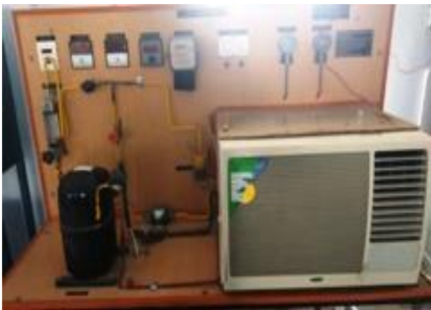
Fig.2 Front side of Window Air Conditioning Trainer
