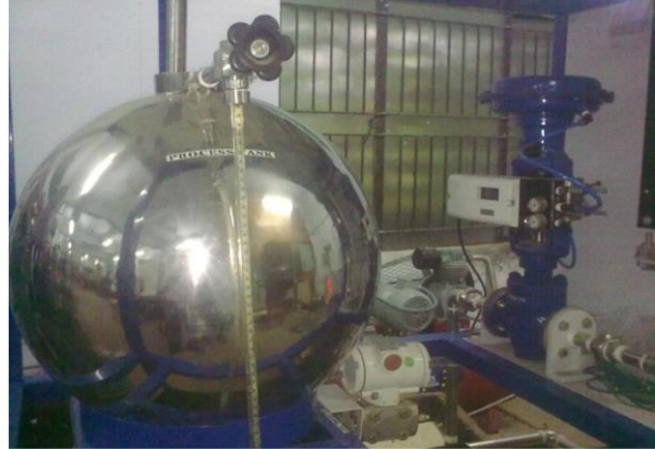
Fig. 5 Experimental Setup of Laboratory Spherical Tank Level Process
