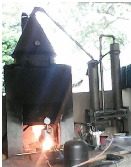
Fig. 2. Steam-atomizing burner integrated with pyrolysis reactor
