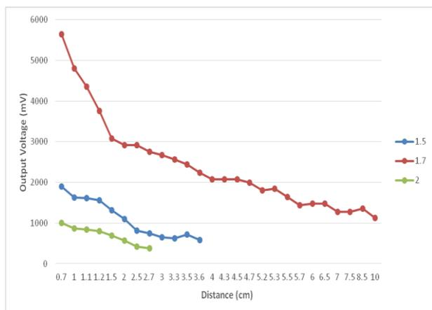
Fig.4: Output Voltage (mV) Vs distance (cm) between two coils at three different frequencies 1.5MHz, 1.7MHz, 2MHz .
