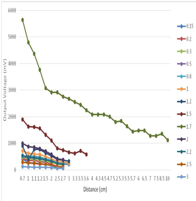
Fig.3: Output Voltage (mV) Vs distance (cm) between two coils at different frequencies(MHz).
