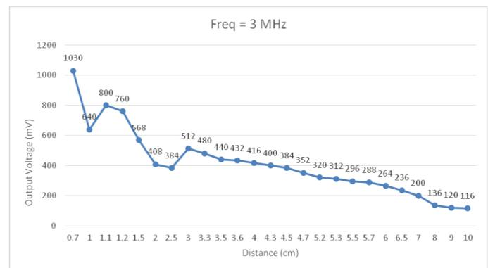
Fig 6: Graph showing Output Voltage generated for 3MHz frequency varying distance between two coils(cm).
