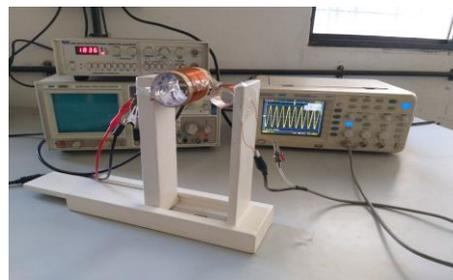
**Fig.2: Setup with transmitter and receiver as solenoid coils.**
