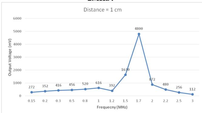
Fig. 5: Output Voltage at different frequencies by keeping distance between two coils as constant i.e. 1 cm.
