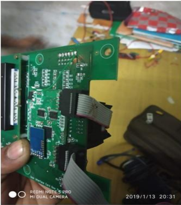
Fig. 22. Bypassing the calibration cable, b. Changing the circuit path by adding cables
