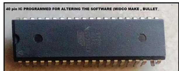
Fig. 8. Microcontroller used for altering the programme in MIDCO, Bullet.
