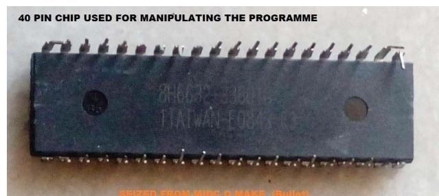
Fig. 9. Microcontroller used for altering the programme in MIDCO, Bullet.
