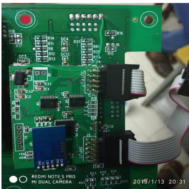
Fig. 12. Bypassing Calibration Cable; b. Chips Soldered to manipulate the circuit path
