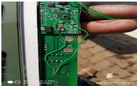
Fig. 19. Changing the chips circuit path by bypassing the cables.
