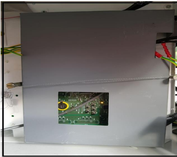
Fig. 4. The Mother board will be sealed in order to prevent the access of the Mother Board for inserting the additional devices. The opening is meant for making the display price alteration whenever there is a change in selling price of the petroleum products.
