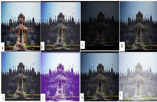
Fig. 2. Temple image under various light illuminations: a) direct sunlight b) indirect sunlight c) High contrast d) Low contrast. The resultant Gamma corrected images are shown in Figure (i) to (l) respectively.
