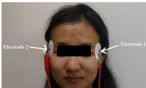
Fig. 5 Electrode placement for acquiring EOG
