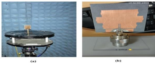
Fig. 4. Proposed antenna (a) In the anechoic chamber (b) Connected to VNA
