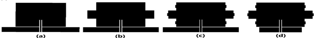
Fig. 2. All iterations of antenna (a) 0 th iteration (b) 1 st iteration (c) 2 nd iteration (d) 2 nd iteration with modified ground width
