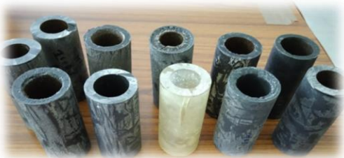
Fig.8: test specimen after compression test.
