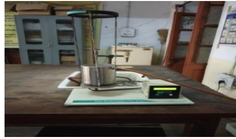
Fig.11: Thermal conductivity test rig (Lees Apparatus).
