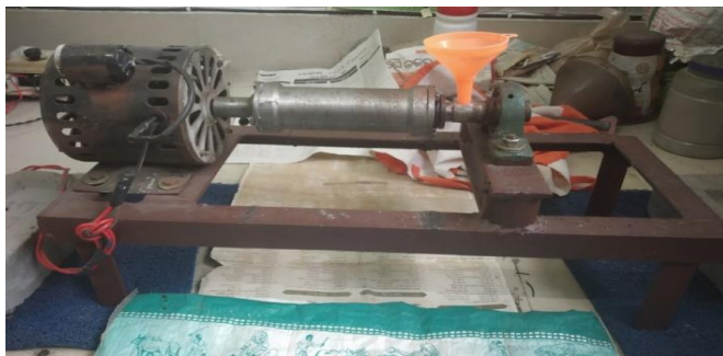
Figure 1: presents Isometric view of the hollow cylinder used in centrifugal casting
