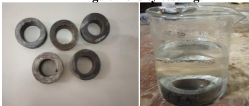
Fig.10: Test specimen in water absorption test.
