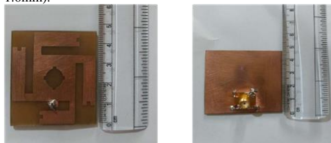
Fig. 6(a) Front view of fabricated (b) Back view of fabricated antenna
