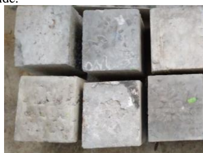
Fig. 2. Ambient curing of cubes.
