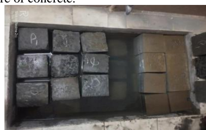
Fig. 3. Water curing of cubes.
