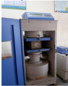
Fig. 4. Compressive strength testing machine.
