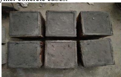
Fig. 1. Preparation of cubes.
