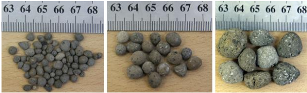
Fig. 1 Expanded clay aggregates: LECA S, LECA M and LECA L (from left to right)
