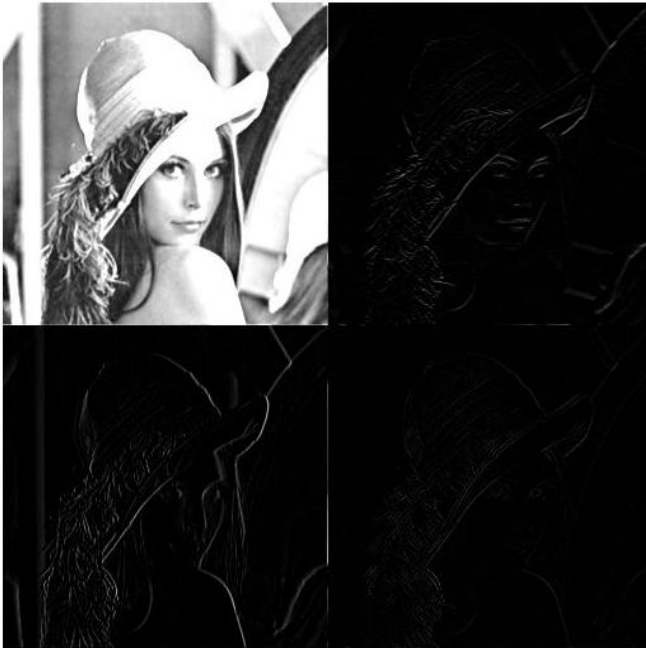
Fig. 5. One level 2-D RDWT decomposition of Lena Image (size of LL, LH, HL, and HH=256x256)
