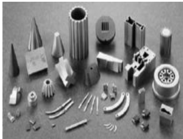
Fig. 1(a). Parts manufactured by EDM [36]
