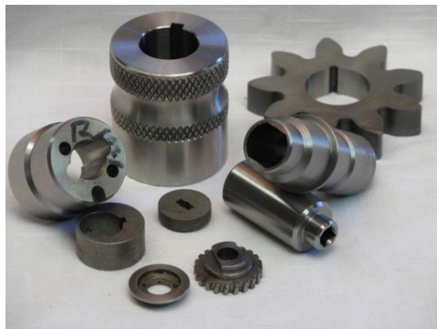
Fig. 1(b). Parts manufactured by EDM [37]
