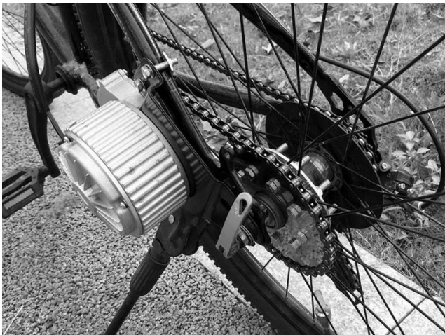
Fig. 3. External motor with chain link (Source: L-faster)
