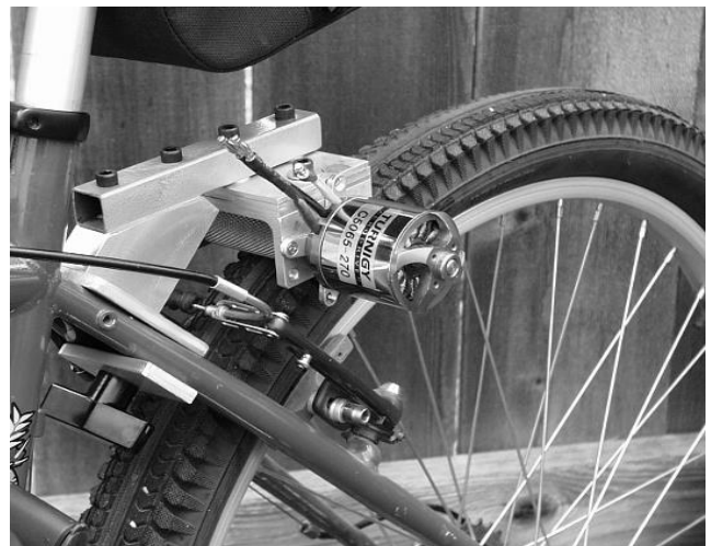
Fig. 5. Frictional motor drive (Source: ebikeschool)
