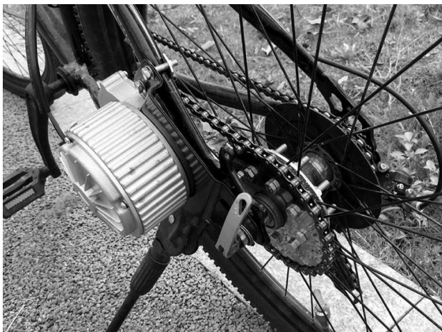
Fig. 3. External motor with chain link (Source: L-faster)
