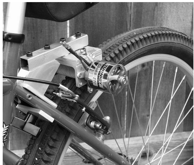
Fig. 5. Frictional motor drive (Source: ebikeschool)
