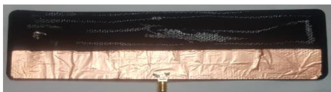
Fig.10. Fabricated flexible antenna on solar cell front view
