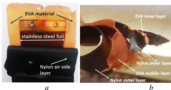
Fig. 2 a) solar cell back view b) layers in encapsulation of a solar cell
