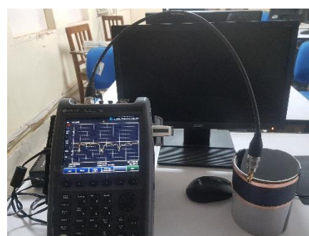
Fig.13. Experimental setup for measuring return loss of the H-plan bending ( r=6\text{cm} ) antenna
