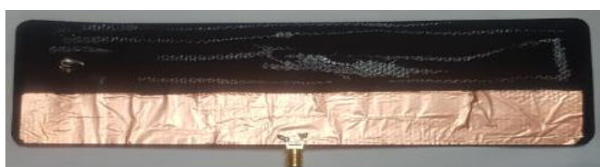
Fig.11. Fabricated flexible antenna on solar cell back view
