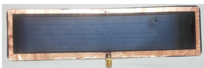
Fig.10. Fabricated flexible antenna on solar cell front view
