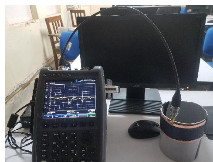
Fig.13. Experimental setup for measuring return loss of the H-plane bending ( r=6\text{cm} ) antenna
