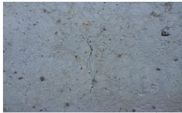
Figs.10 and 11 Initial and final cracks on 15% wet marine brown algae concrete
