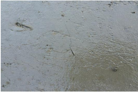
Figs.10 and 11 Initial and final cracks on 15% wet marine brown algae concrete
