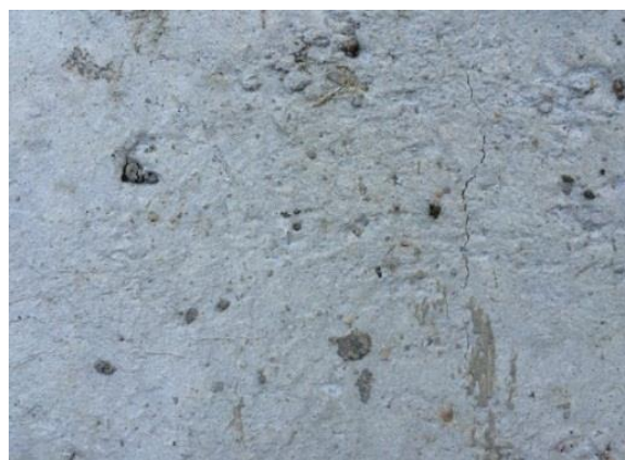
Figs.8 and 9 Initial and final cracks on conventional concrete
