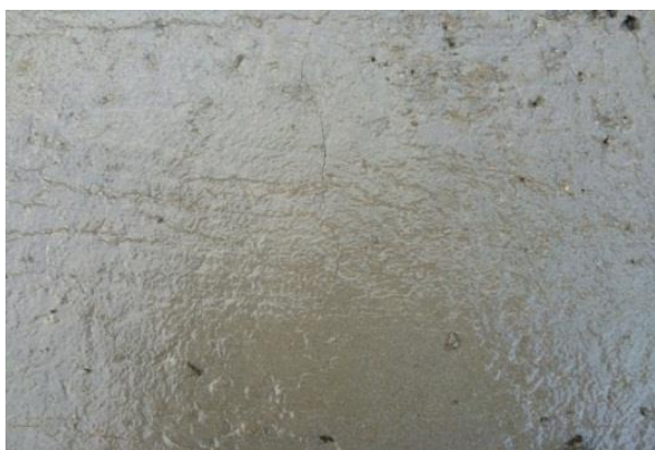
Figs.8 and 9 Initial and final cracks on conventional concrete
