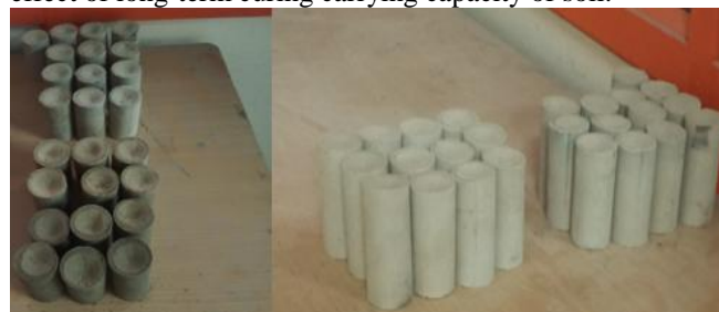
Figure 10: Typical photo of sample preparation for UCS test in different curing time
