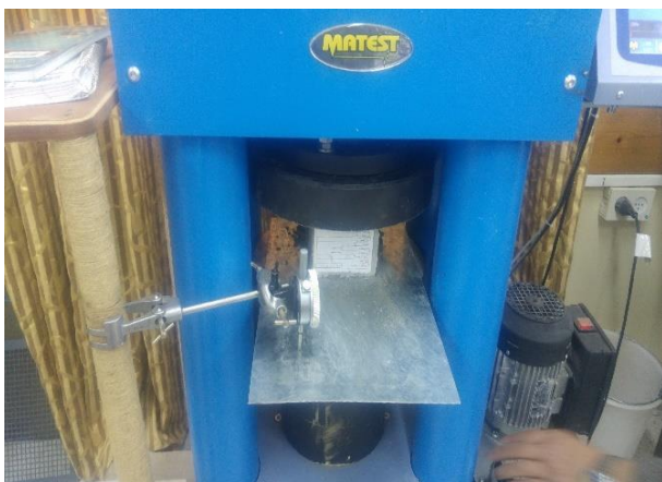
Figure (2) : Setup of compressive test and mode failure of samples made with TTW from NWWTP
