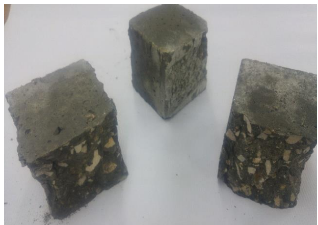
Figure (2) : Setup of compressive test and mode failure of samples made with TTW from NWWTP
