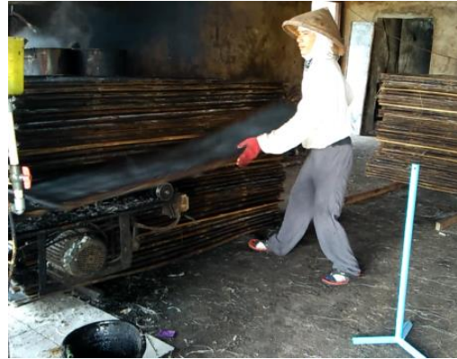
Figure 1. Pressing Work Station with Activities Inserting Zinc into the Press Machine
