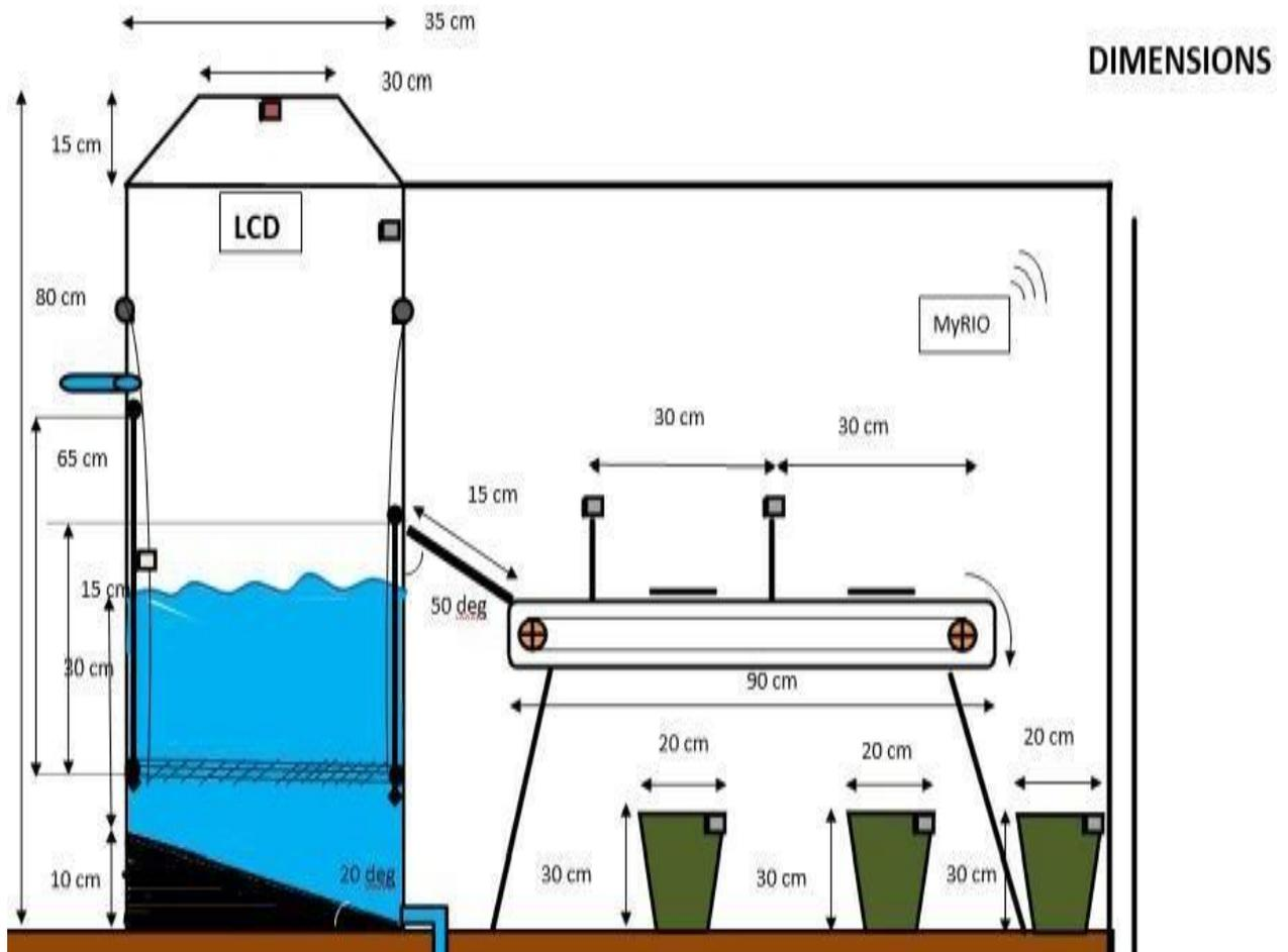
Fig.5 Block diagram of trash bin structure with dimensions
