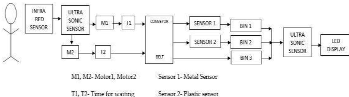
Fig. 1 Block diagram for the control circuit of smart trash bin
