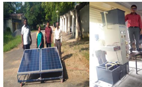
Fig.4.Solar PV water pump Training System
