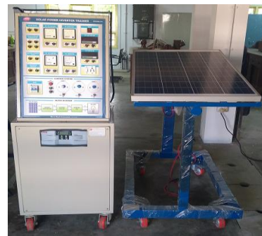
Fig.3.Solar PV Training System
