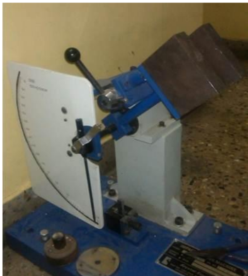
Fig.4. Impact testing of the specimen
