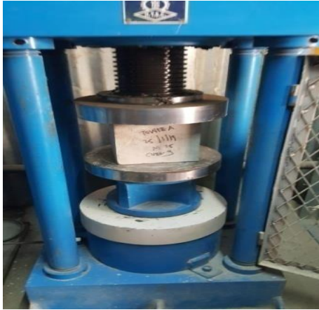
Fig. 2. Testing of concrete cube
