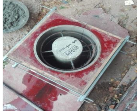
Fig. 4. Reinforcement Details for jacketing along with its Shuttering.
