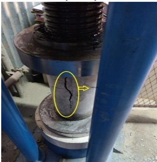
Fig. 3. Failure of concrete cylinder
