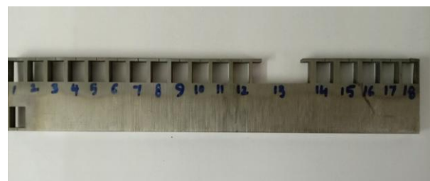
Fig. 3 Titanium grade-5 material after performing on wire cut EDM
