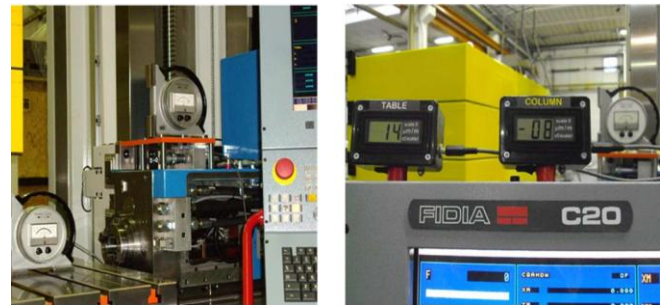
Fig. 14: Inclinometers used to measure roll and pitch
