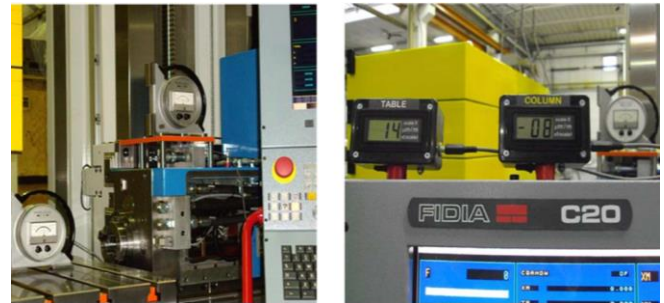
Fig. 14: Inclinometers used to measure roll and pitch
