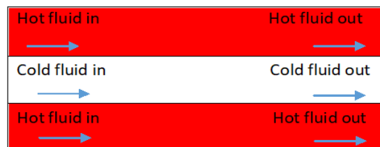
Fig 1. Parallel flow heat exchanger
