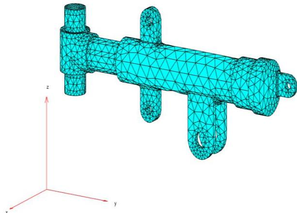
Fig. 6.Generated Mesh with minimum element size of 7
