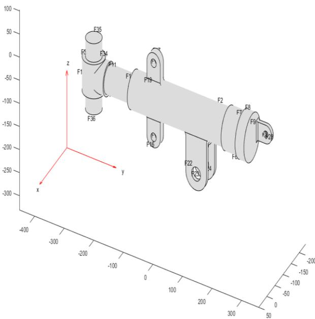
Fig. 2.Landing gear model with face labels
